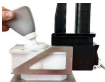
2. Fill tank and screw back lid
